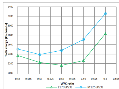
Fig. 16. Effect of W/C ratio on total charge diffused in Coulombs.
